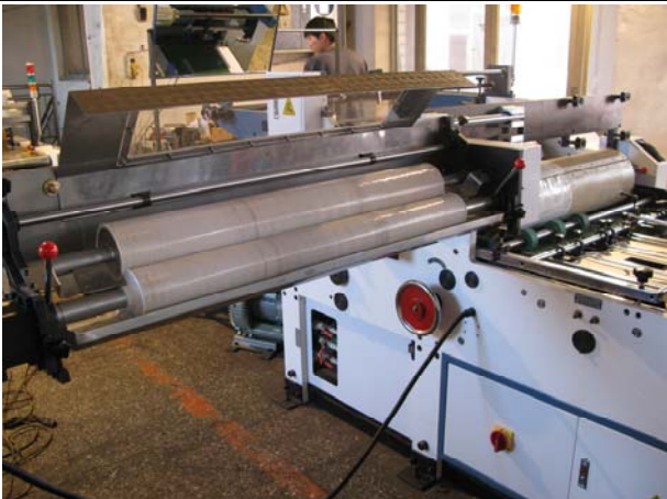
Gluing Part can be pull out for washing
